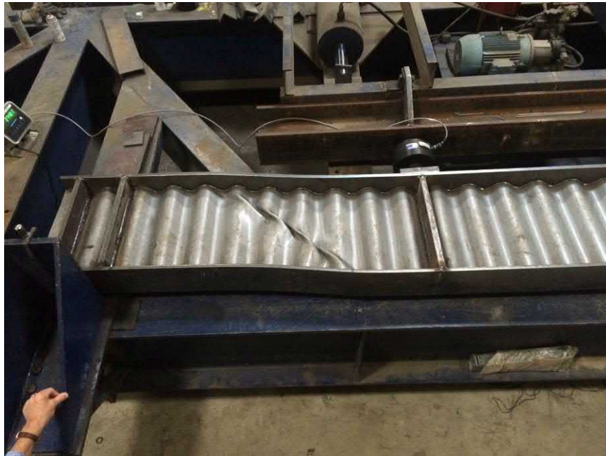
Figure 3 – Typical Shear Failure
