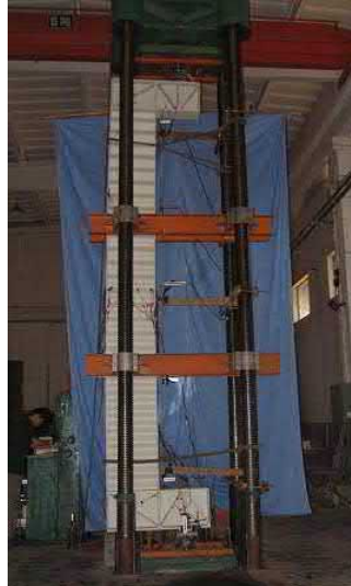
(b) eccentric compression test
