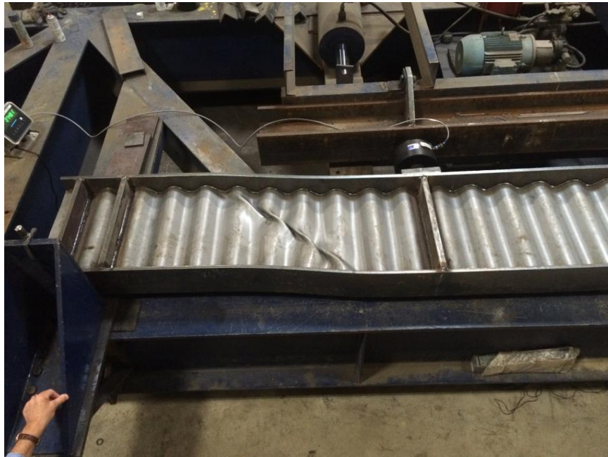
Figure 3 – Typical Shear Failure
